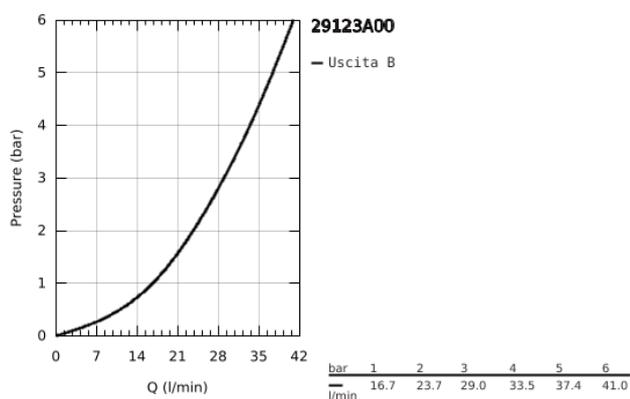
29 123 A00 **GROHTHERM SMARTCONTROL MISCELATORE TERMOSTATICO A 1 VIA**
