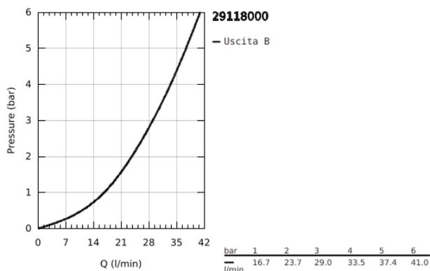
29 118 000 **GROHTHERM SMARTCONTROL MISCELATORE TERMOSTATICO A 1 VIA**
